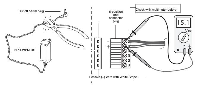
Fig. 8. Adapting a NPB-WPM-US wall mount AC adapter to power the WEB/CP-700.
